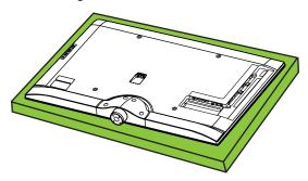
2 Hook the slot in the base onto the tab on the stand column, then push the base into place.
